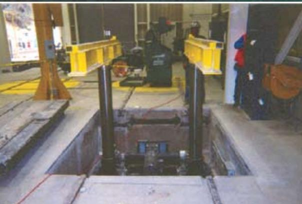
Macton Truck Repair Hoists increase shop productivity and safety by allowing shop personnel to perform maintenance, repair and inspection of rail vehicles that are elevated at a convenient height above the shop floor.
